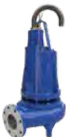
NE - Cast Iron body, multi-purpose pump, double mechanical seal, discharge nozzle up to 6", semi-open impeller.
