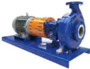
CPP - Single Stage end suction horizontal centrifugal pump, enclosed impeller, radially split casing with flanged connections.
