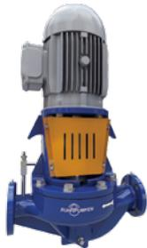
IVP - Split-coupling, flanged suction and discharge on common centerline, up to 350 psi, fully enclosed, impeller with hydraulic balance which prevents vibration, radially splitcase.
