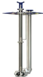
VSP - Single Stage single suction vertical centrifugal pump, volute type case, flanged and threaded discharge, cast iron casing, flexible coupling.
