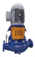
replacement of the mechanical seal becomes fast and simple, without disconnecting the pump from the pipeline or removing the motor (Not available for IVP-CC). Options exist to select between internally or externally mounted mechanical seal, which allows choice between high performance or economical seals. The IVP Pump comes in 28 hydraulic sizes.
