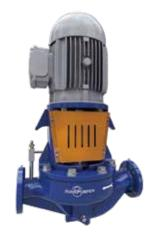
replacement of the mechanical seal becomes fast and simple, without disconnecting the pump from the pipeline or removing the motor (Not available for IVP-CC). Options exist to select between internally or externally mounted mechanical seal, which allows choice between high performance or economical seals. The IVP Pump comes in 28 hydraulic sizes.
