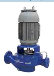
The IIL pumps meet the requirements of ANSI B73.2. The integral one-piece unit, suitable for in-line pedestal mounting has fully enclosed, balanced, one-piece design impellers. The casing has flanged suction and discharge on common centerline and its top pull-out design simplifies maintenance.
