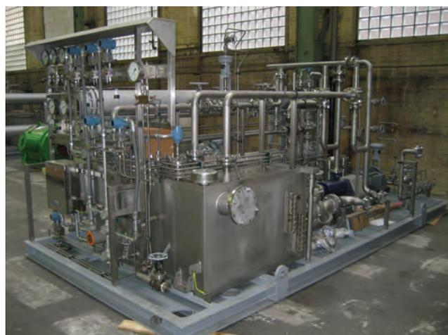
Jet Pump Unit and Lube Oil System, ready to pack and ship
