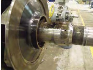
*Impeller and stage casing – coker debris present.*
