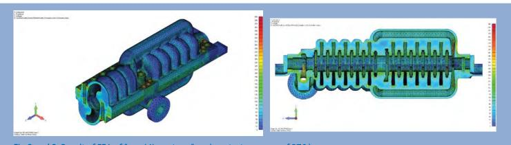
Fig 2 and 3. Result of FEA of "von Mises stress" under a test pressure of 276 bar.
