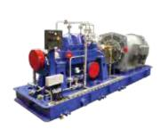
SM - Axially split, horizontal multi-stage, centrifugal pump, near-centerline mounted, single suction, radial, closed impeller (API Type BB3).
