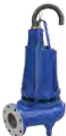
NE - Cast Iron body, multi-purpose pump, double mechanical seal, discharge nozzle up to 6", semi-open impeller.
