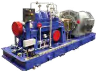
SM - Axially split, horizontal multi-stage, centrifugal pump, near-centerline mounted, single suction, radial, closed impeller (API Type BB3).
