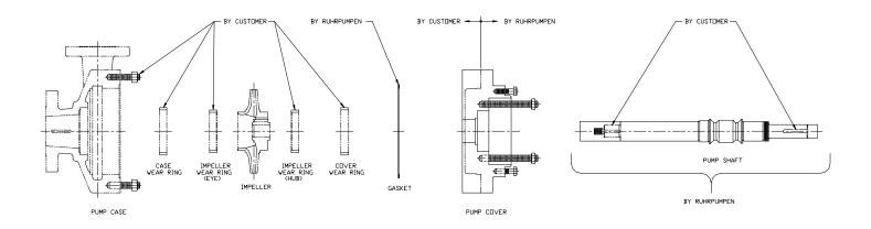
Customer to repair pump in their facility. Ruhrpumpen to provide the following:
