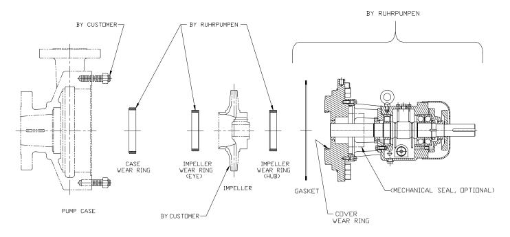
Customer to repair pump in their facility. Ruhrpumpen to provide the following:
