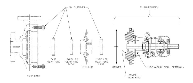
Customer to repair pump in their facility. Ruhrpumpen to provide the following:
