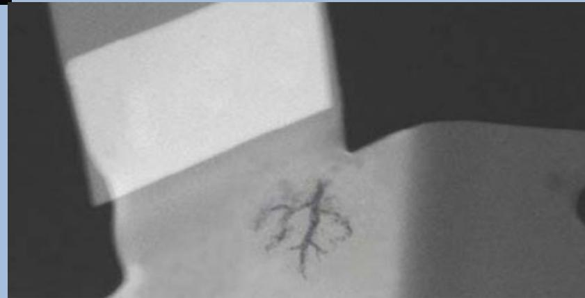
Examples of casting defects such as shrinkage & tears
