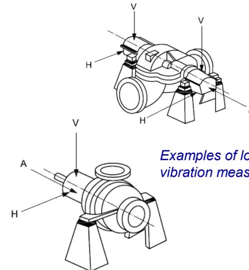
Examples of location of vibration measurements
