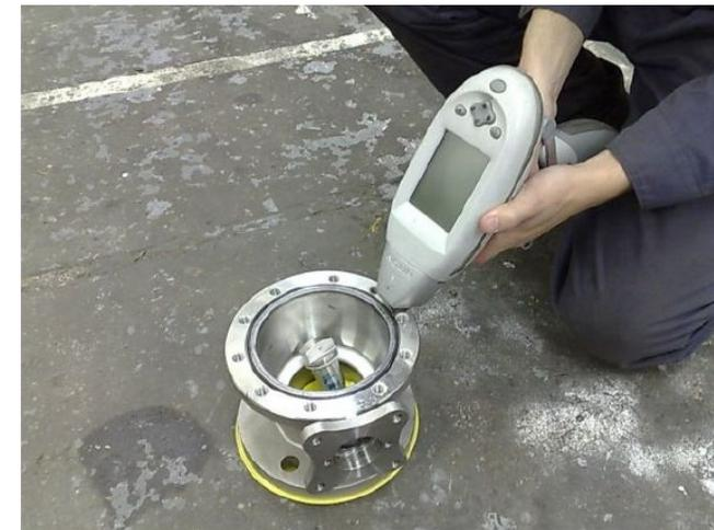
Example of testing with hand-held XRF analyzer
