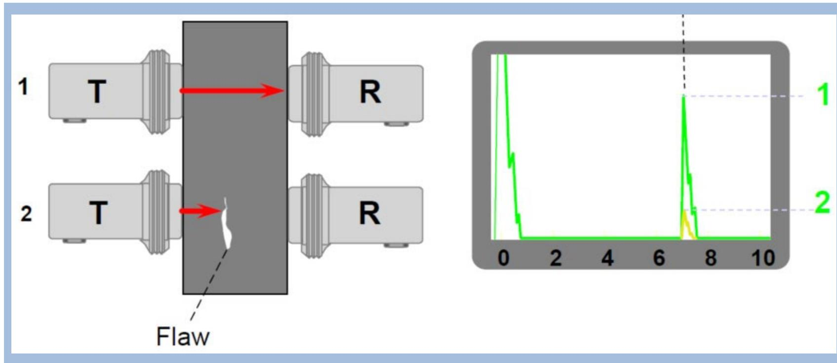
The above plot, shows another illustration of the **Attenuation** (2 Probe) technique.
