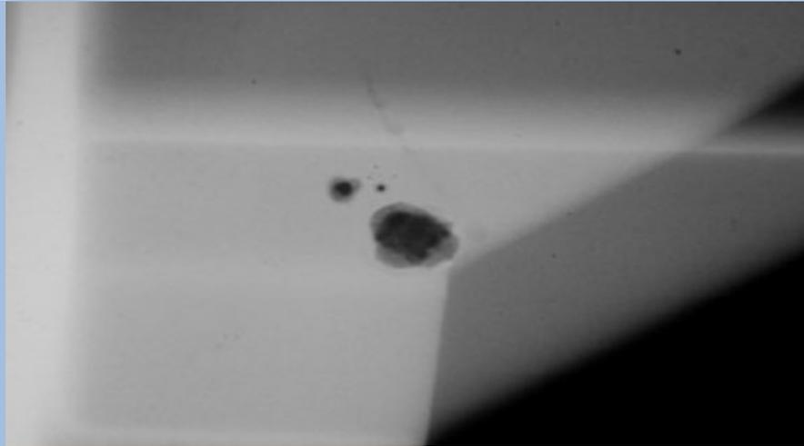
Examples of casting porosity being detected
