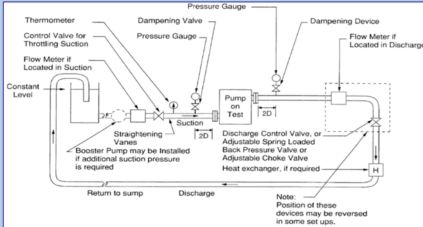
A schematic of a typical Test Bed setup, as shown in the Hydraulic Institute standards.
