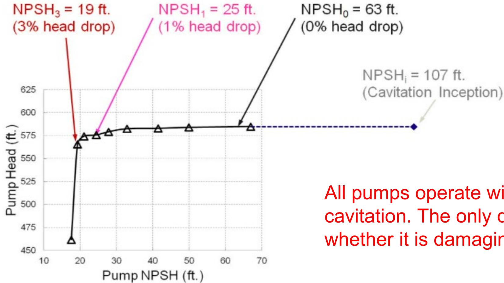
All pumps operate with suction cavitation. The only question is whether it is damaging cavitation.
