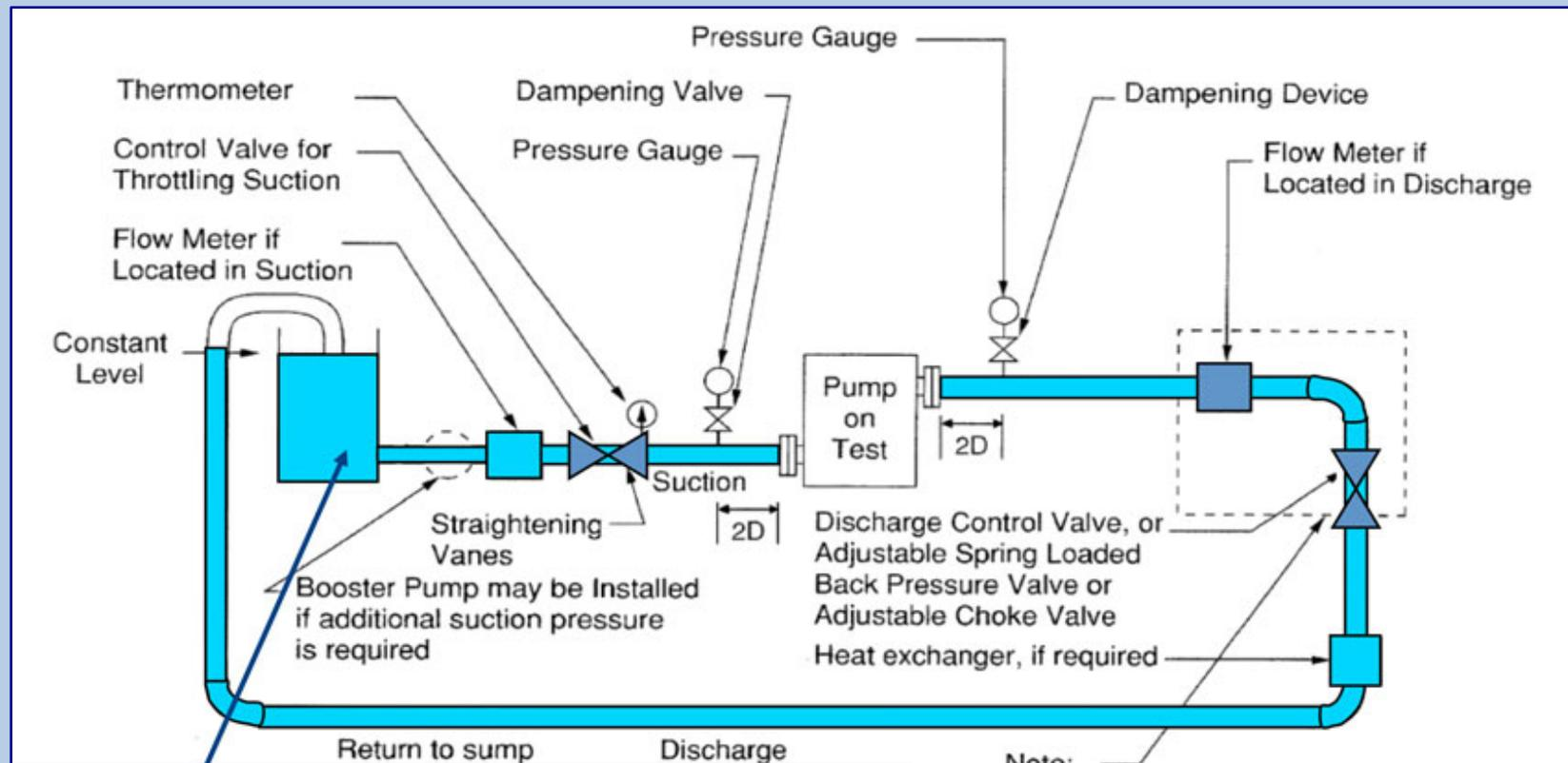
The water then returns to the Tank or Sump in the case of Vertical pumps.
