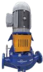
IVP - Rigid-coupling, flanged suction and discharge on common centerline, up to 350 psi, fully enclosed, impeller with hydraulic balance which prevents vibration, radially splitcase. Fire Service, Air Conditioning Systems, Condensed Water, Ice Water, Service Water, Ocean Water, Building Water Supply Systems.
