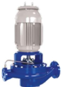
IIL - Back pull-out design, CI/SS impeller, packing box cover, casing-flanged suction, front wear rings, manual vent plug.
