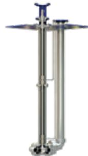
VSP - Single Stage single suction vertical centrifugal pump, volute type case, flanged and threaded discharge, cast iron casing, flexible coupling. Sump Drainage, Flood Control, Air Wash Systems, Power Plants, Chemical Industry, Municipal Systems, Water Treatment, Process Plants, Sewage Lift Stations.
