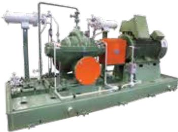
Axially split, horizontal single or two stage, double volute casing, double suction, closed impeller. Heavy duty process design according to API 610 latest edition. Pipeline Service-Mainline and Booster, Oil Extraction, Refinery, Chemical, Petrochemical, Metallurgical Industry, and Power Stations.
