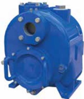
Self Priming Pump, easy maintenance without the need of disconnecting piping, easy access to impeller and seal, availability of mounting above the liquid being pumped, designed to allow up to 3 inch diameter solids. Steel, Paper Mills, Mining, Food Processing, Power Plant, Automotive, Wineries.
