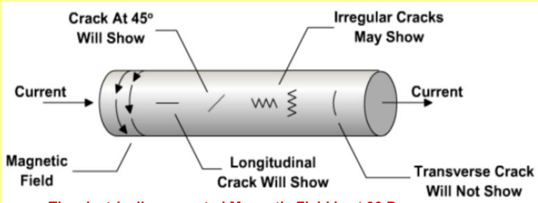
**The electrically generated Magnetic Field is at 90 Degrees to the Current Flow Direction.**
