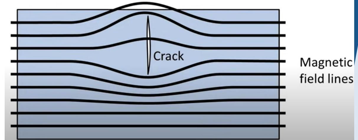
If the piece is free from flaws the magnetic field lines run within the piece and parallel. If there is a crack at or near to the surface, the magnetic field lines will locally leave the surface and a local leakage field occurs.
