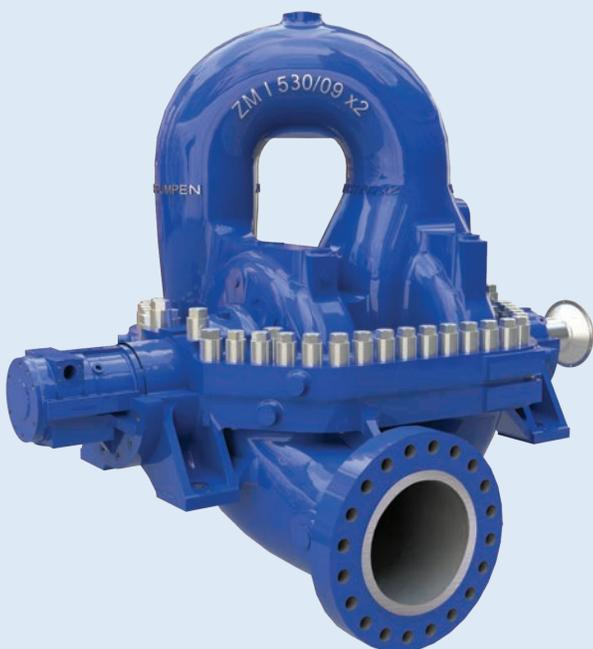
Our ZM pump range of axially split case centrifugal pumps has a heavy-duty process design according to API 610 latest edition (BB1 type) for applications in the oil and gas industry such as the extraction of oil (land and offshore), as mainline and booster pumps in hydrocarbon pipelines, and different applications in refineries, tank farms and petrochemical plants.
