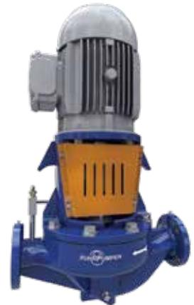
The replacement of the mechanical seal becomes fast and simple, without disconnecting the pump from the pipeline or removing the motor (Not available for IVP-CC). Options exist to select between internally or externally mounted mechanical seal, which allows choice between high performance or economical seals. The IVP Pump comes in 28 hydraulic sizes.
