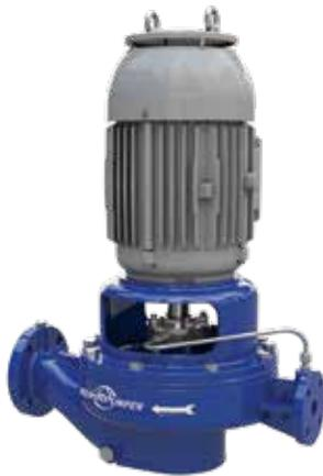
The IIL pumps meet the requirements of ANSI B73.2. The integral one-piece unit, suitable for in-line pedestal mounting has fully enclosed, balanced, one-piece design impellers. The casing has flanged suction and discharge on common centerline and its top pull-out design simplifies maintenance.
