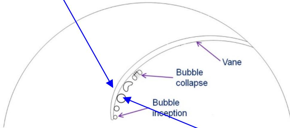
NPSH Cavitation Damage appears on front side (suction side) of vane
