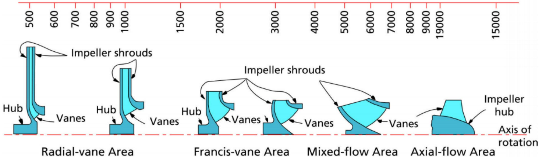
$$N_S = N_{(RPM)} Q_{(BEP \text{ Full Dia})}^{0.5} / H_{(BEP \text{ Full Dia})}^{0.75}$$
