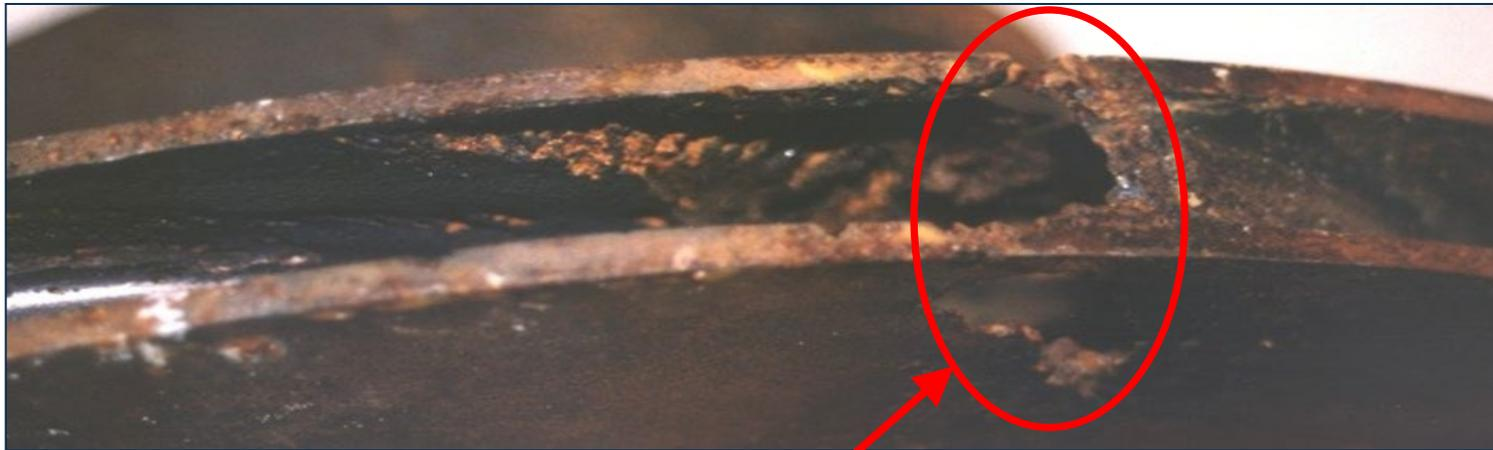
The central core of the Discharge Recirculation Vortex, is such a low pressure that the liquid starts to vapourise & as the bubbles move to the outer area of the vortex, where the pressure is much higher, they Cavitate (implode) against the Impeller Shrouds, and cause the hole damage shown.
