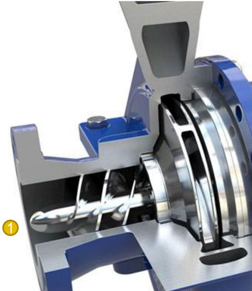
1 **NPSH<sub>r</sub>** of a pump can be significantly reduced by using an inducer
