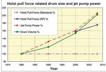
Fig. 2. Hoist pull force related to drum size and jet pump power.
