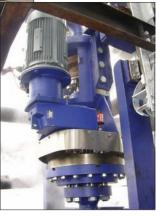
Figs. 3. and 4. Electrical driven decoking hoist (left hand and right hand version) and electrical driven drill stem drive.
