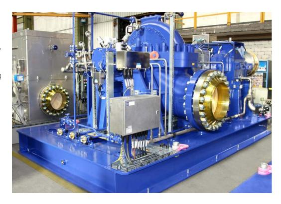
Both of the pumps—type ZLM I 530/08—have a flow of 24,656 GPM and a head of 1657 feet with a rated power of 10,326 HP. The pumps were successfully tested at our German manufacturing plant and have already been delivered to the client. They are expected to be installed by the end of this year and put into pretest operation in March, 2014.
